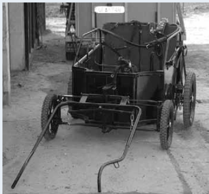
Photo 1a: The wheelchair-buggy, designed to be pulled by one horse
