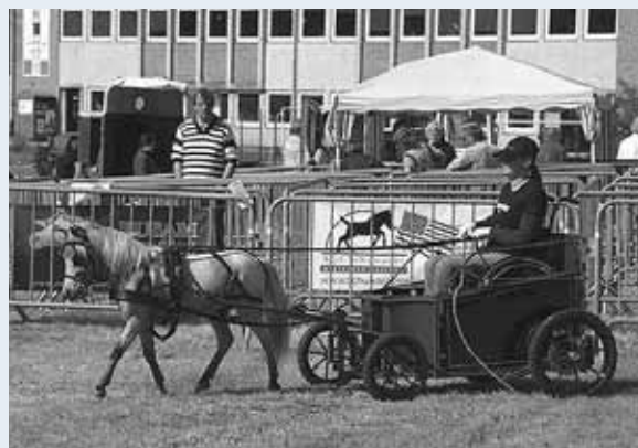
Photo 1b: The buggy is about 20 cms above the ground, 160 cms long, and 105 cms wide
